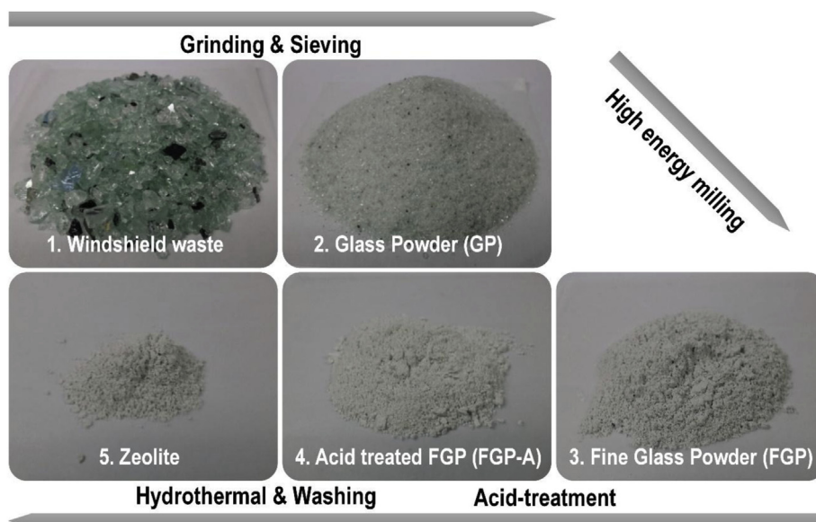
Fig. 1. Flowchart with powder pictures for the synthesis of A-type zeolite.
