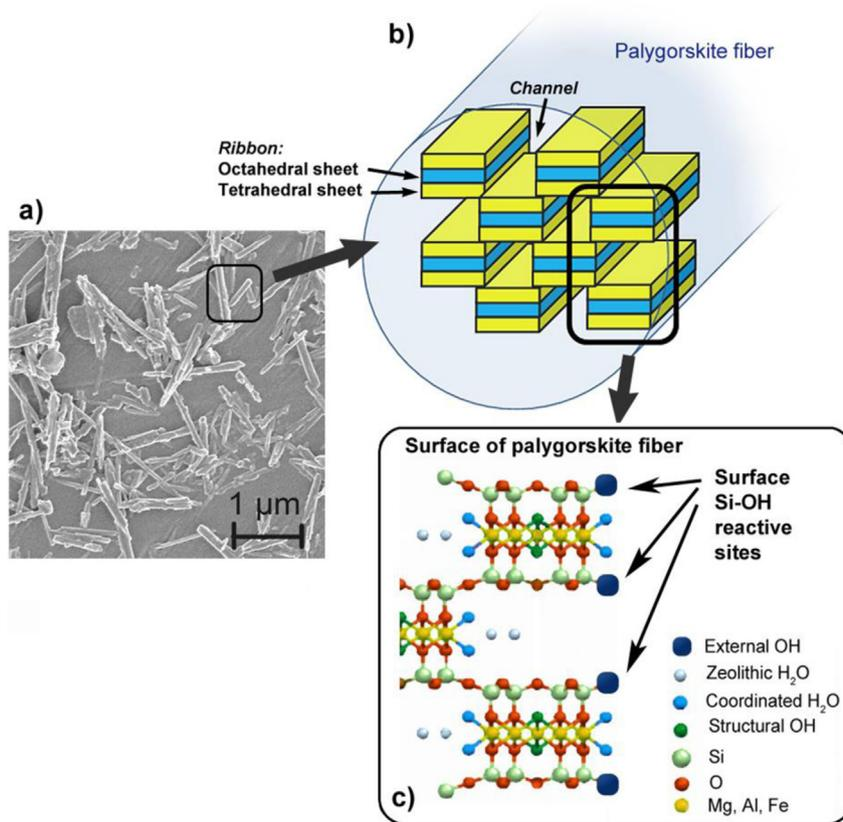
**Fig. 1.** Multi-scale description of the structure of palygorskite clay: (a) SEM micrograph of  $\text{Na}^+$  exchanged purified palygorskite ( $\text{Na}^+\text{-Pal}$ ), (b) Schematic overview of ribbons and channels, (c) orojection on (001) plane of the crystallographic structure showing the Si–OH reactive sites.
