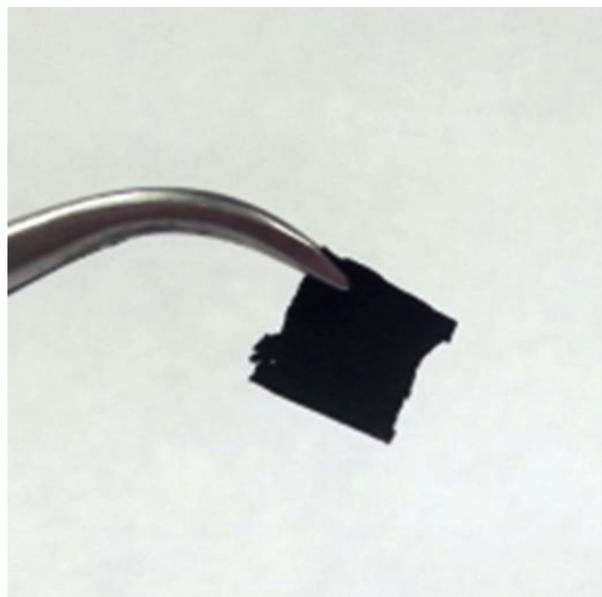
Fig. 1. The binder-free, free-standing film consisting of  $\text{Fe}_2\text{O}_3$  NP-deposited fCNT.
