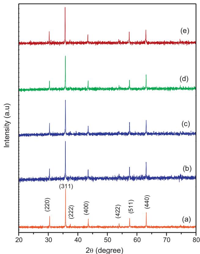
Fig. 1. XRD pattern of (a) S1, (b) S2, (c) S3, (d) S4 and (e) S5 samples of  $\text{NiFe}_2\text{O}_4$  prepared at  $900^\circ\text{C}$  for 3 h.
