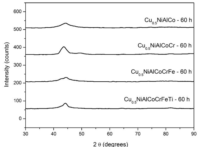
**Fig. 2.** XRD patterns of amorphous MA quaternary Cu<sub>0.5</sub>NiAlCo to septenary Cu<sub>0.5</sub>NiAlCoCrFeTi powders after milling for 60 h.
