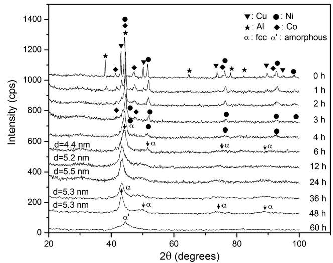
**Fig. 1.** XRD patterns of MA quaternary Cu<sub>0.5</sub>NiAlCo powders with different milling times.
