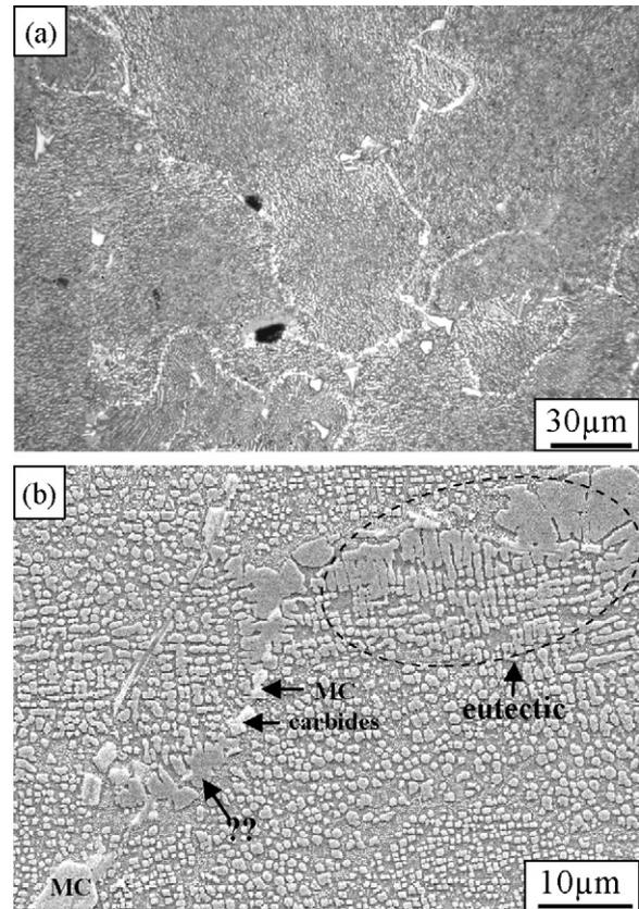
**Fig. 2.** Micrographs of the blade after 25,000 h of service exposure at high temperatures showing (a) the inherent casting defects and (b) the decoration of grain boundaries with  $\gamma'$  and MC carbides.
