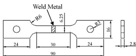
**Fig. 1.** Schematic diagram showing the dimensions of laser-welded specimens used in tensile tests.
