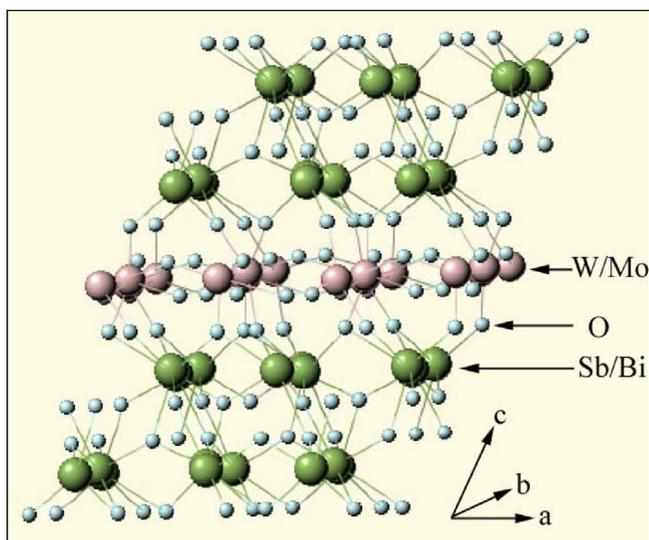
**Fig. 1.** Schematic depiction of  $A_2BO_6$  ( $A = \text{Sb, Bi}$  and  $B = \text{W, Mo}$ ) possessing Aurivillius structure.
