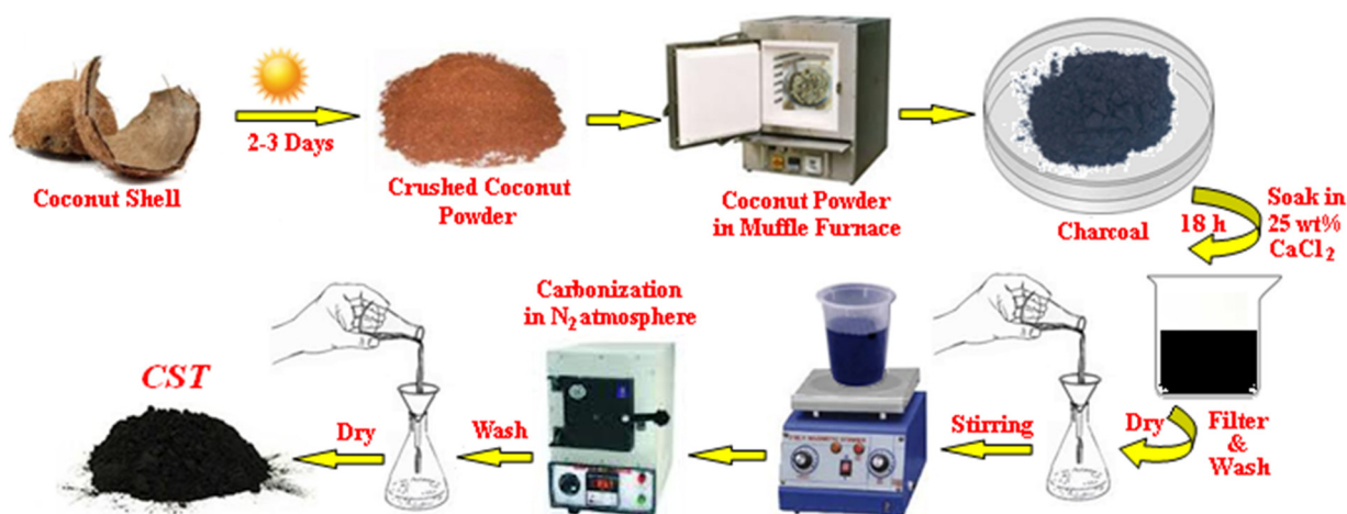
Fig. 1. Schematic flowchart for the CST preparation.
