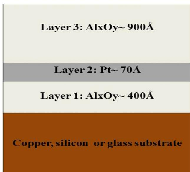
**Fig. 1.** Schematic diagram of the  $\text{Al}_x\text{O}_y$ -Pt- $\text{Al}_x\text{O}_y$  absorber coating deposited on Cu, Si and corning glass substrates.
