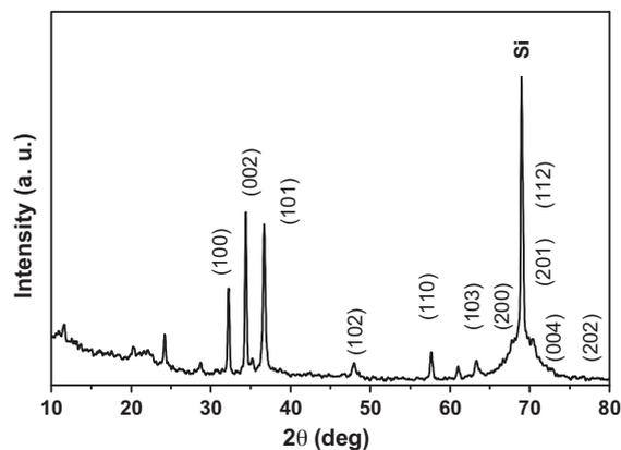
Fig. 1. XRD pattern of as-grown GaN micro-pyramids on Si substrate.
