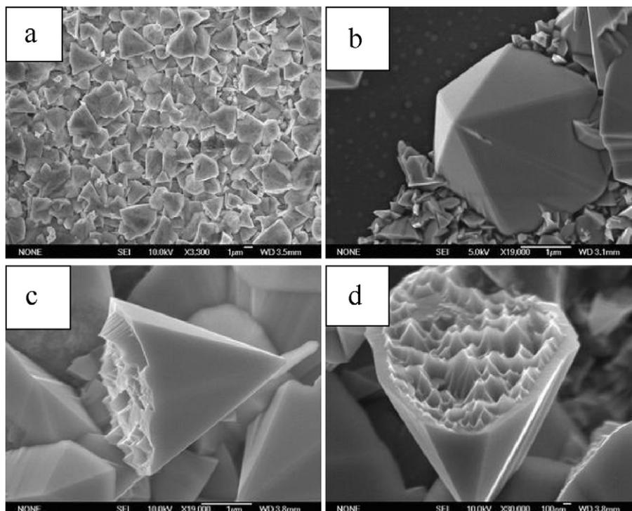
Fig. 2. (a) Low-magnification SEM image of GaN micro-pyramids; (b–d) representative SEM images of GaN micro-pyramids randomly grown on Si substrate.
