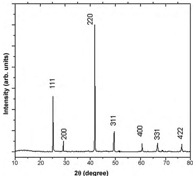
Fig. 2. XRD spectra of GaSb crystals.
