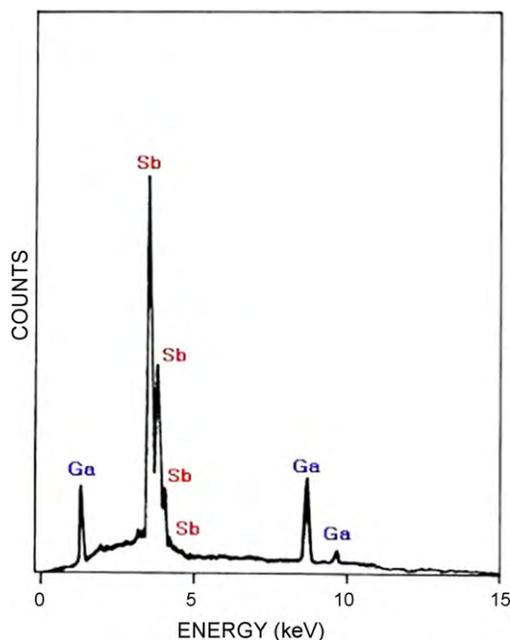
Fig. 1. EDX spectrum of GaSb.
