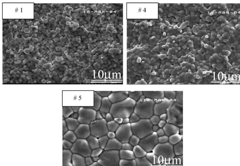
Fig. 1. SEM pictures of the surface of pellets pressed at 4000 bar and sintering at 1000 °C for 20 h. Samples # are indicated according to Table 1.
