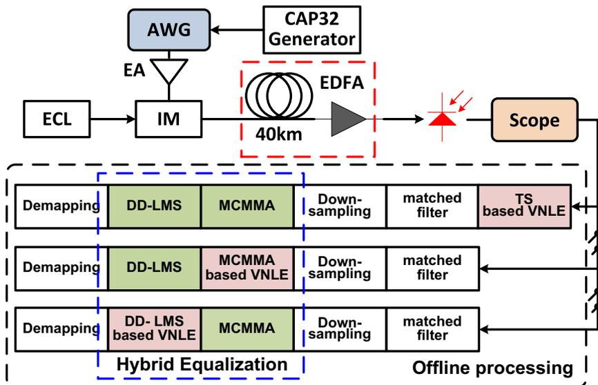
Fig. 2. Experiment setup of CAP32 transmission system using different VNLE schemes, ECL: external cavity laser, IM: intensity modulator, EA: electrical amplifier, AWG: arbitrary waveform generator.
