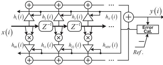
Fig. 1. Structure of Volterra based nonlinear equalization.
