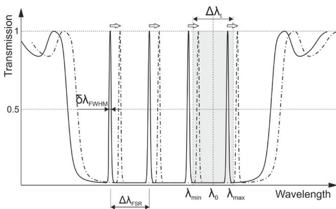
(b) Transmission Spectrum of the DBR Sensor
