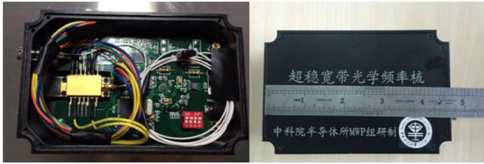
Fig. 1. The integrated ultra stable wideband OFC (left: the inside of OFC; right: the integrated OFC generator).
