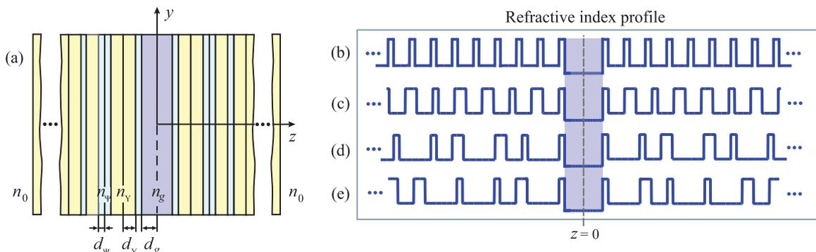
Fig. 1. (a) The schematic of a symmetrical Bragg reflection waveguide that consists of a core layer sandwiched between two aperiodic mirrors. Index profiles of the waveguide's cladding where layers are arranged according to the generation rules of (b) periodic, (c) Fibonacci, (d) Thue–Morse, and (e) Kolakoski sequences.
