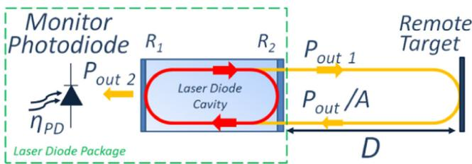
Fig. 1. Basic scheme of a self-mixing interferometer.
