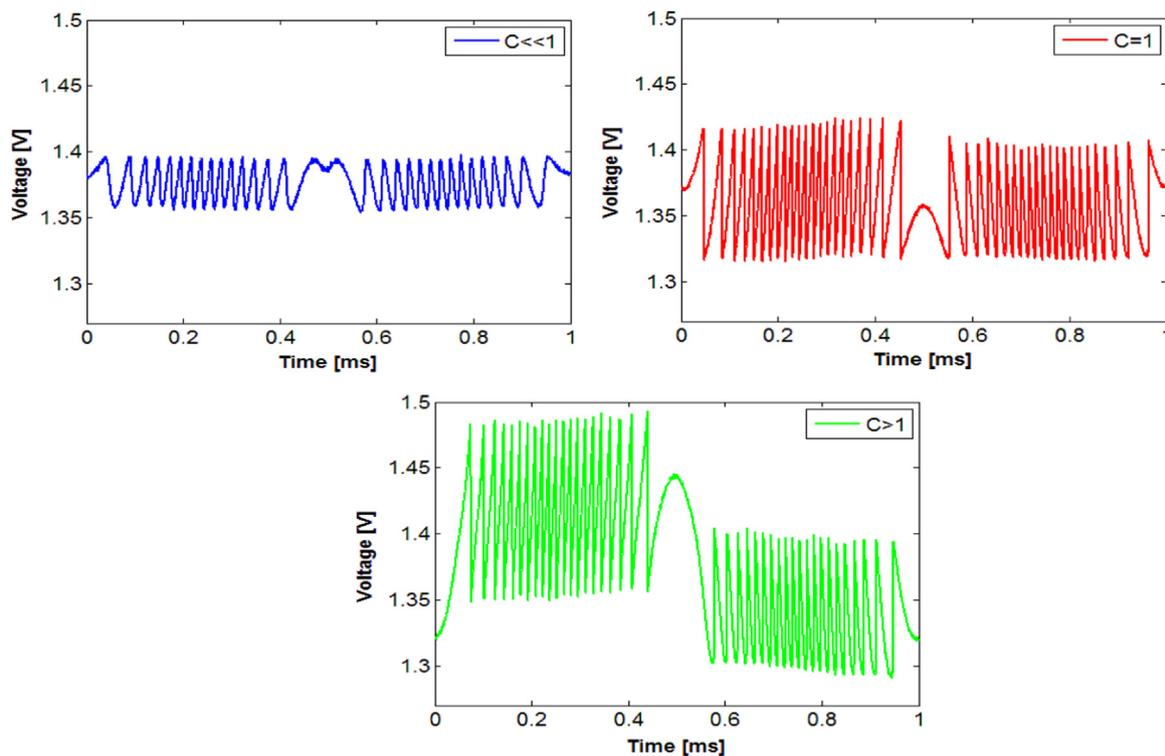
Fig. 2. Self-mixing signal in correspondence to a sinusoidal displacement, as a function of  $C$ .
