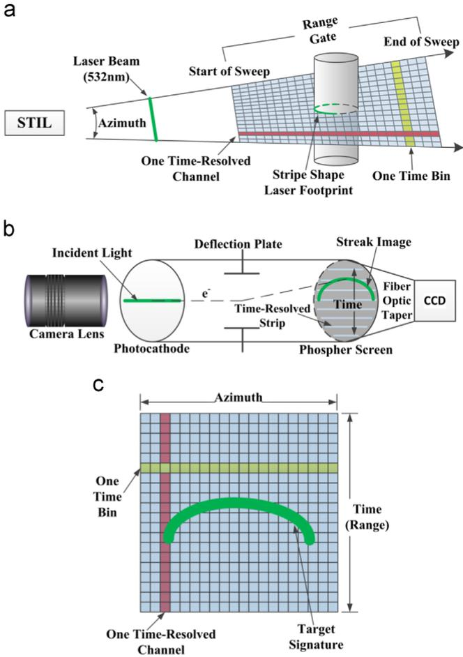
**Fig. 1.** (a) Schematic diagram of the streak tube imaging lidar data collection process. (b) Illustration of the work principle of the streak tube detector. (c) The streak image at the phosphor screen, as captured by CCD.
