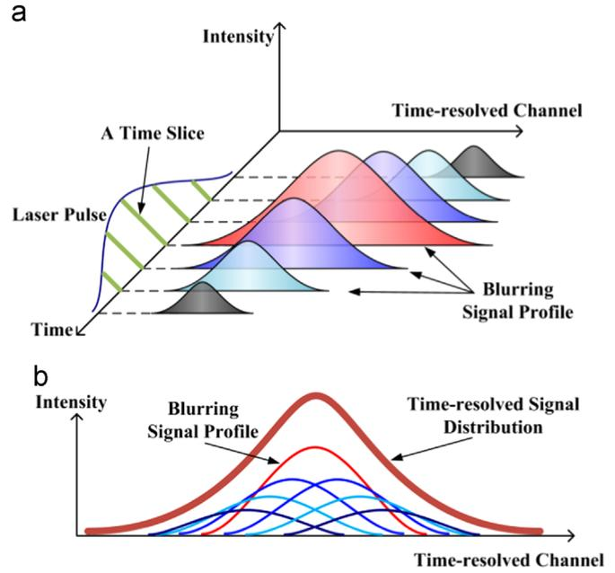
**Fig. 2.** The composition of the time-resolved signal. (a) The laser energy in each time slice generates a corresponding blurring signal with different peak positions in the time-resolved channel. (b) The time-resolved signal is formed by integrating all of the blurring signals.
