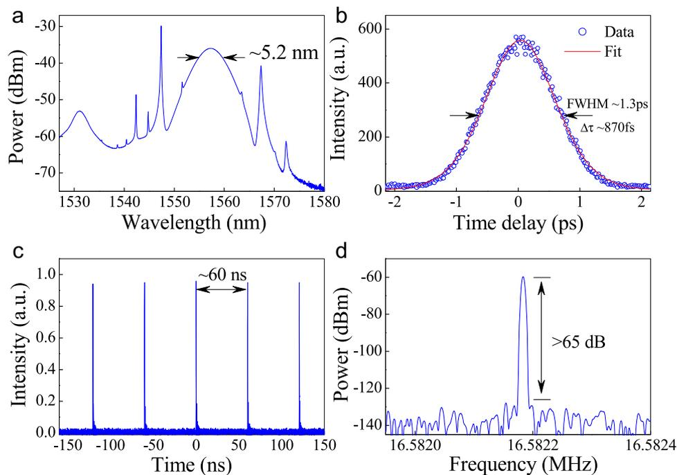
**Fig. 2.** Experimental results of CSs at 1557 nm. (a) Optical spectrum, (b) autocorrelation trace, (c) oscilloscope trace, and (d) fundamental RF spectrum of the laser outputs.
