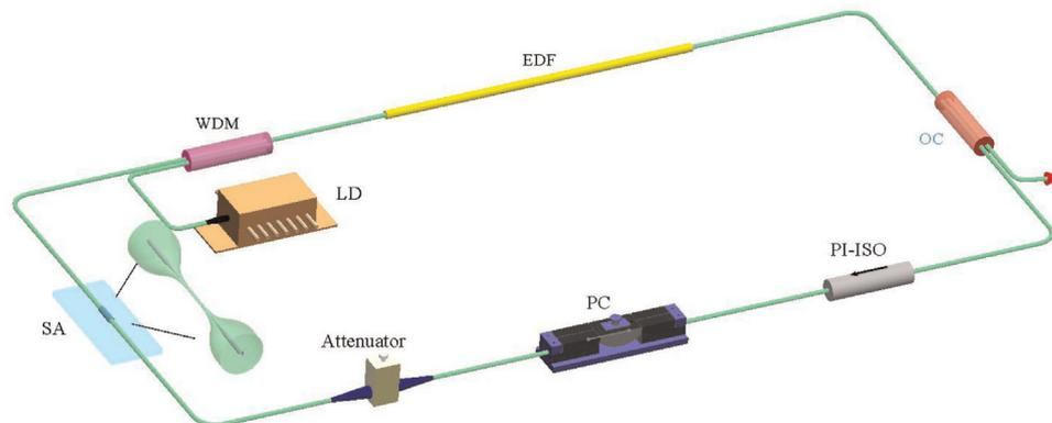
**Fig. 1.** Experimental setup of the proposed all-fiber laser. LD, laser diode; WDM, wavelength-division multiplexer; EDF, erbium-doped fiber; OC, optical coupler; PI-ISO, polarization-independent isolators; PC, polarization controller; SA, saturable absorber.
