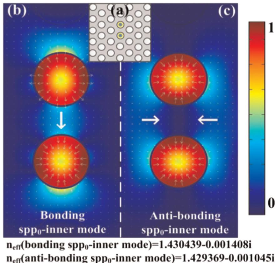
**Fig. 1.** The (a) cross section of the two adjacent gold-coated layers embedded in a finite hexagonal air hole lattice, and the electric field distribution of the (b) bonding  $spp_0$ -inner mode and (c) anti-bonding  $spp_0$ -inner mode at 1550 nm when  $n_0=1.52$ . The arrows represent the directions of the local transverse electric fields.
