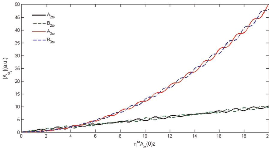
Fig. 1. The amplitudes of the harmonic waves under the double resonance phase-matching conditions  $\Delta k_1 = \kappa_{2\omega}$  and  $\Delta k_2 = \kappa_\omega - \kappa_{2\omega} + \kappa_{3\omega}$ .
