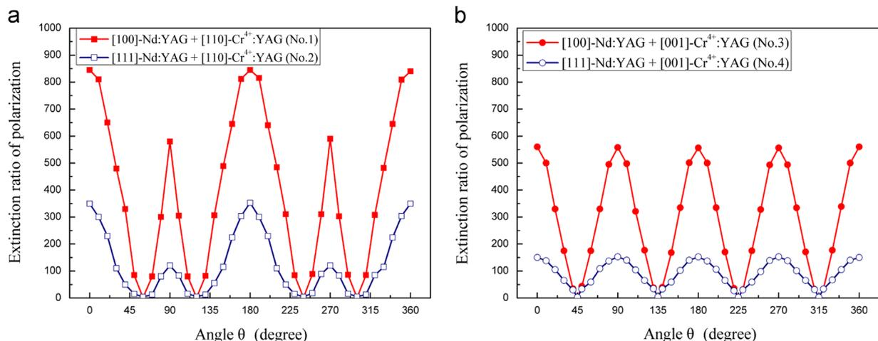
Fig. 2. The extinction ratio of output polarization as a function of angle  $\theta$  for of passively Q-switched Nd:YAG/ $\text{Cr}^{4+}$ :YAG lasers four combinations. (a)  $[100]$ -Nd:YAG +  $[110]$ - $\text{Cr}^{4+}$ :YAG (No. 1) and  $[111]$ -Nd:YAG +  $[110]$ - $\text{Cr}^{4+}$ :YAG (No. 2); (b)  $[100]$ -Nd:YAG +  $[001]$ - $\text{Cr}^{4+}$ :YAG (No. 3) and  $[111]$ -Nd:YAG +  $[001]$ - $\text{Cr}^{4+}$ :YAG (No. 4).
