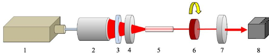
Fig. 1. Experimental setup of passively Q-switched laser. (1. Laser diode; 2. Focus lens; 3. Half wave plate; 4. High reflection coating, HR@1064 nm, AR@808 nm; 5.  $[111]$ - and  $[100]$ -cut Nd:YAG rod; 6.  $[001]$ - and  $[110]$ -cut  $\text{Cr}^{4+}$ :YAG crystal; 7. Mirror, transmission is 55%; 8. Power meter.  $[111]$ - and  $[100]$ -cut Nd:YAG rod are used as the gain medium,  $[001]$ - and  $[110]$ -cut  $\text{Cr}^{4+}$ :YAG crystal are used as the saturable absorber, respectively.)
