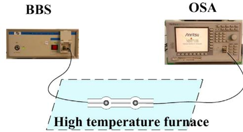
Fig. 3. Experimental setup.
