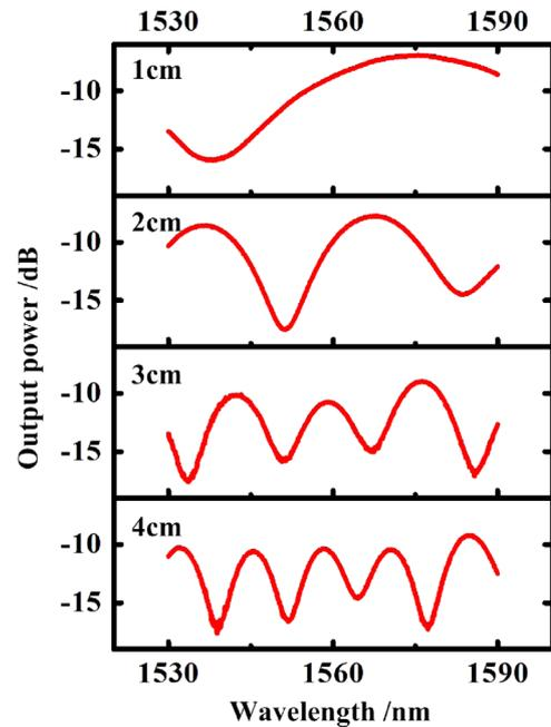
Fig. 4. Transmission spectra of the proposed MZI sensor with different  $L$ .
