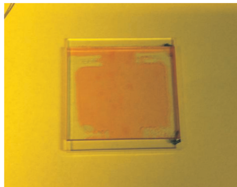
Fig. 1. Cell with spacers of 20 \mu\text{m} filled with E7 LC mixture doped with MR.
