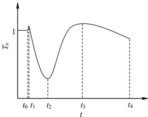
Fig. 1. General transmitted light relaxation curve of ferrofluids under a centripetal gradient magnetic field.
