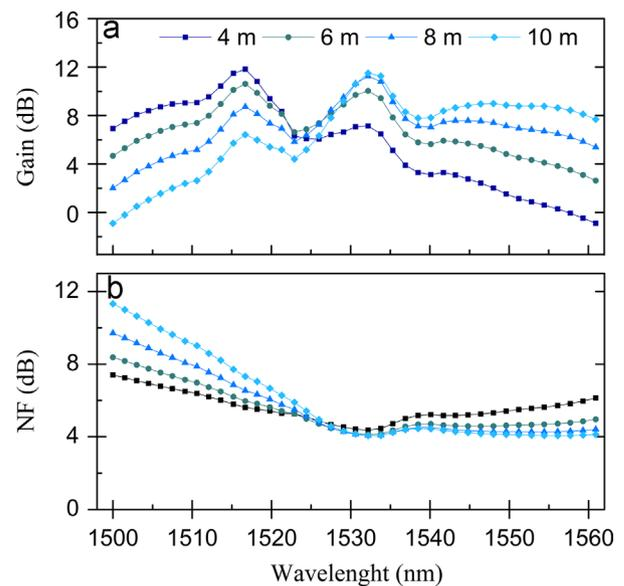
Fig. 2. Gain (a) and NF (b) wavelength dependency after 80 km transmission for different EDF lengths and a pump wavelength of 1412 nm and fixed power of 800 mW.
