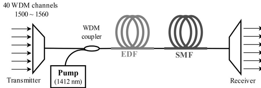
Fig. 1. Schematic diagram of the proposed hybrid amplifiers.
