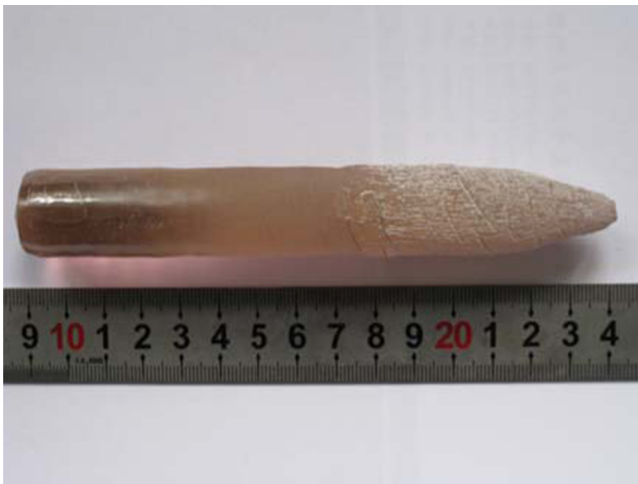
Fig. 1. Photograph of the as-grown Er:GYSGG laser crystal.
