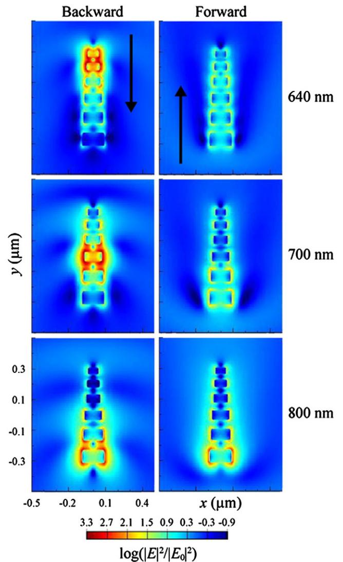
**Fig. 2.** Shift of the electric field enhancement within a dipole-array antenna (DA6) depending on the direction of incidence and the wavelength of the plane wave. The electric field is normalized to the incident plane wave. Antenna parameters are  $N = 6$ ,  $r = 1.14$ ,  $\sigma = 0.4$ ,  $AR = 2.1$ ,  $a_3 = 120$  nm.
