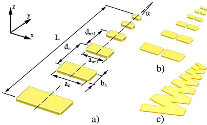
**Fig. 1.** Geometrical configuration of log-periodic antennas (a) dipole array, (b) gap-dipole array and (c) zigzag antenna.
