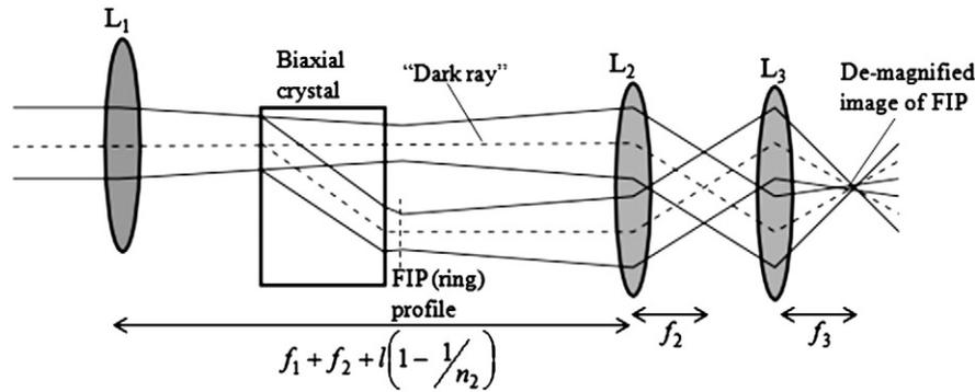
Fig. 1. The optical setup used to form a ring shaped beam at the focal plane of the objective  $L_3$ .
