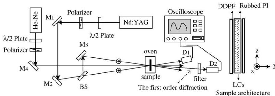
Fig. 2. The experimental setup and the configuration of sample cell.
