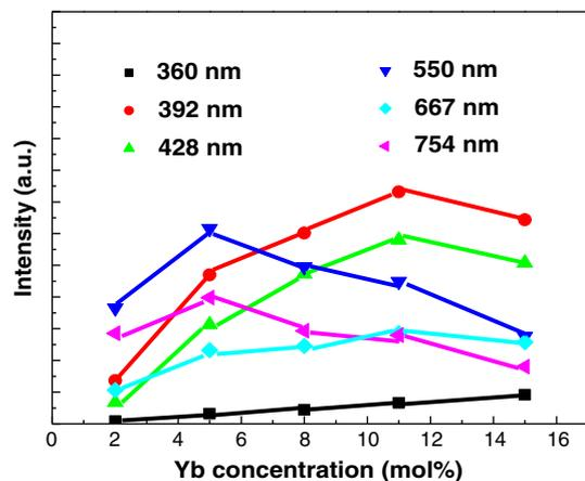
Fig. 3. Intensity of the UC emissions peaked at 362, 392, 428, 550, 667 and 754 nm as a function of  $\text{Yb}^{3+}$  concentration.
