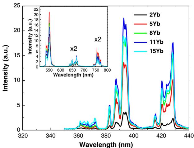
Fig. 2. Measured UV and violet UC emissions in 0.1 mol%  $\text{Ho}^{3+}/x$  mol%  $\text{Yb}^{3+}:\text{Y}_2\text{O}_3$  ( $x=2, 5, 8, 11, 15$ ) bulk ceramics under 976 nm diode laser excitation. The inset is the visible and NIR UC emissions of 0.1 mol%  $\text{Ho}^{3+}/x$  mol%  $\text{Yb}^{3+}:\text{Y}_2\text{O}_3$  ( $x=2, 5, 8, 11, 15$ ) bulk ceramics under the same excitation.
