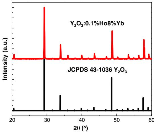
Fig. 1. Measured x-ray-diffraction spectrum of  $\text{Y}_2\text{O}_3$  ceramic doped with 1 mol%  $\text{Ho}^{3+}$  ions and 8 mol%  $\text{Yb}^{3+}$  ions.
