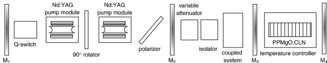
Fig. 2. Schematic of the experimental setup.
