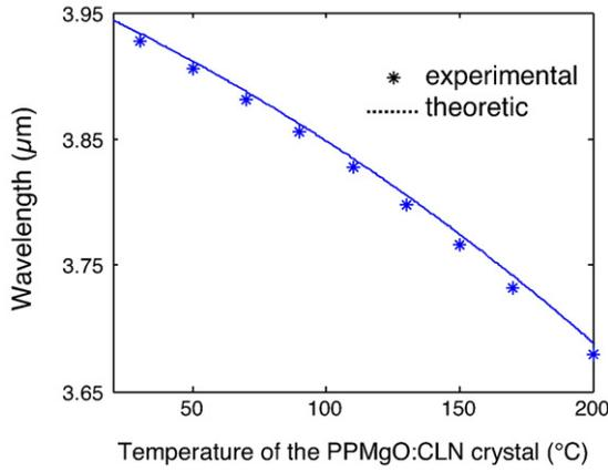
Fig. 1. Laser output wavelength versus temperature of PPMgO:CLN pumped by a 1064 nm laser.
