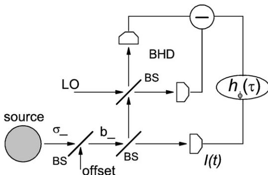
**Fig. 1.** Sketch for conditional homodyne detection. Balanced homodyne detection (BHD) of a quadrature  $E_\phi(\tau)$  is made on the cue of photon detections  $I(t)$ . LO is the local oscillator beam and BS are beam splitters.
