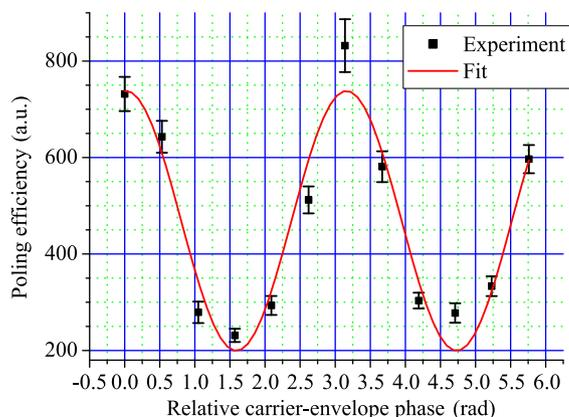
**Fig. 2.** All-optical poling efficiency as a function of relative carrier-envelope phase. Line shows a theoretical fit with  $A + B \cos 2(\phi + \phi_0)$ .  $A = 470$ ,  $B = 270$ . The error bar of each point represents the standard deviation of parameter for each fitting of the SHG intensity in the each experimental run with linear increase with time.
