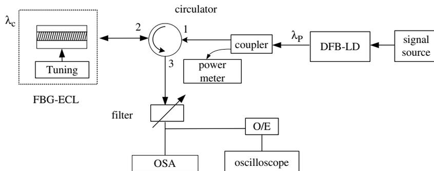
Fig. 1. Experimental setup for wavelength conversion.
