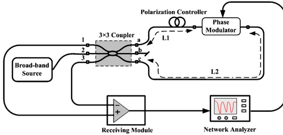
Fig. 1. Topology of negative tap photonic notch filter using a  $3 \times 3$  coupler based Sagnac loop.
