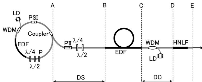
Fig. 1. Schematic diagram of experimental setup. DS: Dispersion shifter between the oscillator and an EDF, DC: Dispersion compensator between an EDF and a HNLF, WDM: Wavelength division multiplexing coupler, PSI: Polarization sensitive isolator, PII: Polarization independent isolator,  $\lambda/4$  and  $\lambda/2$ : quarter and half lambda wave plates, P: Polarizer, HNLF: Highly nonlinear fiber.
