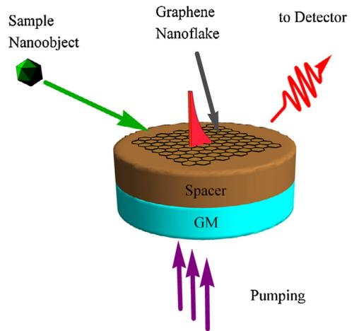
Fig. 1. Schematic picture of graphene spaser based sensor.
