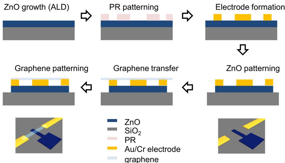
Fig. 1. Schematic of the hybrid device fabrication.
