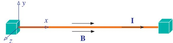
Fig. 1. A current-carrying slender microbeam immersed in a longitudinal magnetic field.
