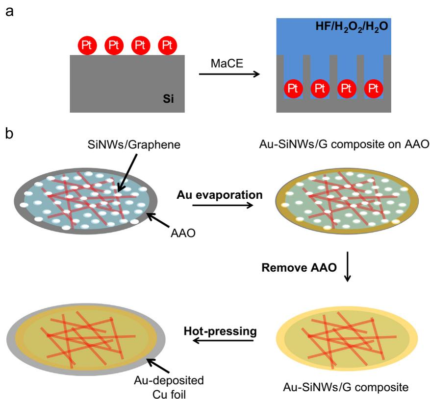
Fig. 1. (a) Schematic formation of SiNWs via Pt-induced etching process. (b) Fabrication process of the Au–SiNWs/G composite anode.
