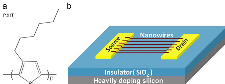
Fig. 1. (a) Chemical structure of P3HT polymer and (b) The schematic diagram of OFET based on P3HT ordered nanowire.
