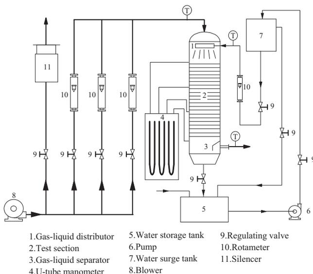
Fig. 1. Sketch of experimental setup and air–water flow loop.
