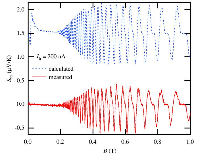
**Fig. 2.** Transverse thermopower  $S_{yx}$  measured directly (solid line) and that calculated from the measured  $\rho_{xx}$  and  $\rho_{yx}$  using Eq. (5) (dotted line), at  $T = 40 \text{ mK}$ . The latter is offset by  $1.5 \mu\text{V/K}$  for clarity.
