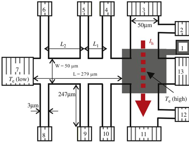
**Fig. 1.** Schematic diagram of the sample. Hatched rectangles are the ohmic contacts. Main (horizontal, from 7 to 13) Hall bar ( $50 \times 279 \mu\text{m}^2$ ) contains three pairs of voltage probes (4–6, 8–10). Secondary (vertical, from 3 to 11) Hall bar ( $170 \times 50 \mu\text{m}^2$ ) is employed as the heater; the voltage probes (2,11) are used for the SdH measurement. A (gray) shaded rectangle is a metallic front gate to control the resistance of the area to be heated.
