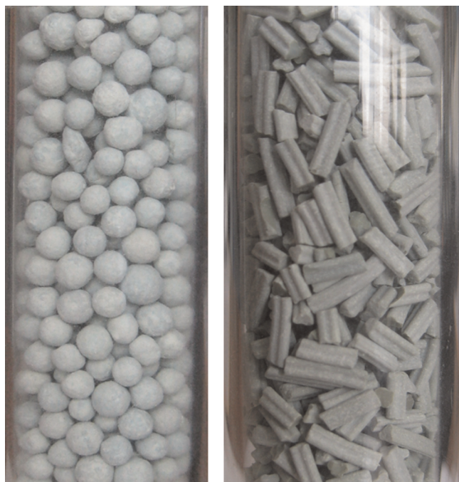
Fig. 1. Left: Sample of spherical beads with near spherical shape and various diameter (around 2 mm)-Right: Sample of trilobed extrudates with various length (around 3 mm). Glass container internal diameter: 16 mm.
