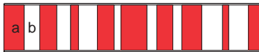
Fig. 1. Schematic for 1D random system. The red area denotes scatterers with gain. The blank is the free space.
