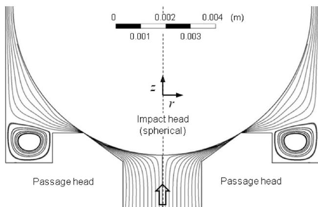
Fig. 1. The geometry of the high pressure homogenizer.
