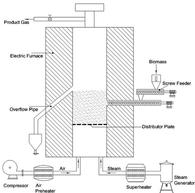
Fig. 1. Schematic diagram of the bubbling fluidized bed biomass gasifier.
