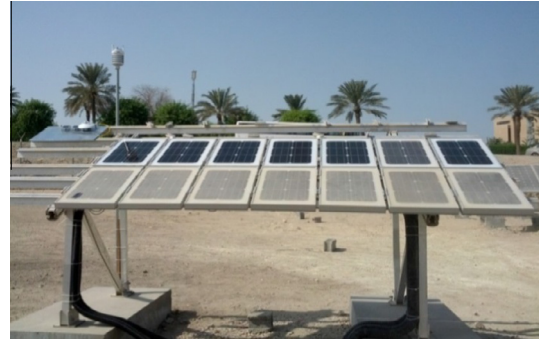
Fig. 1. PV modules test facility at Center of Research Excellence in Renewable Energy (CoRE-RE) – KFUPM.
