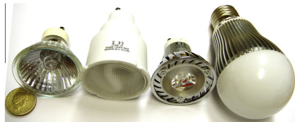
Fig. 1. Typical illumination sources, from left to right: 20 W incandescent lamp, 11 W CFL lamp, 1 W white light LED lamp, 6 W RGB colour-controllable LED lamp.
